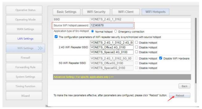
Remark 3: After VONETS device sets the WAN port to access the WiFi hotspot in the routing mode, its LAN port IP is still 192.168.254.254, and the terminal device also obtains the IP address of the same network segment, can login configuration page by 192.168.254.254 or http://vonets.cfg.
