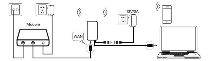
• The VONETS device is used as a wireless router, and the WAN port can be set to connect to a WiFi hotspot and used as a secondary router. Its Ethernet port and Ethernet cable are both LAN ports.
