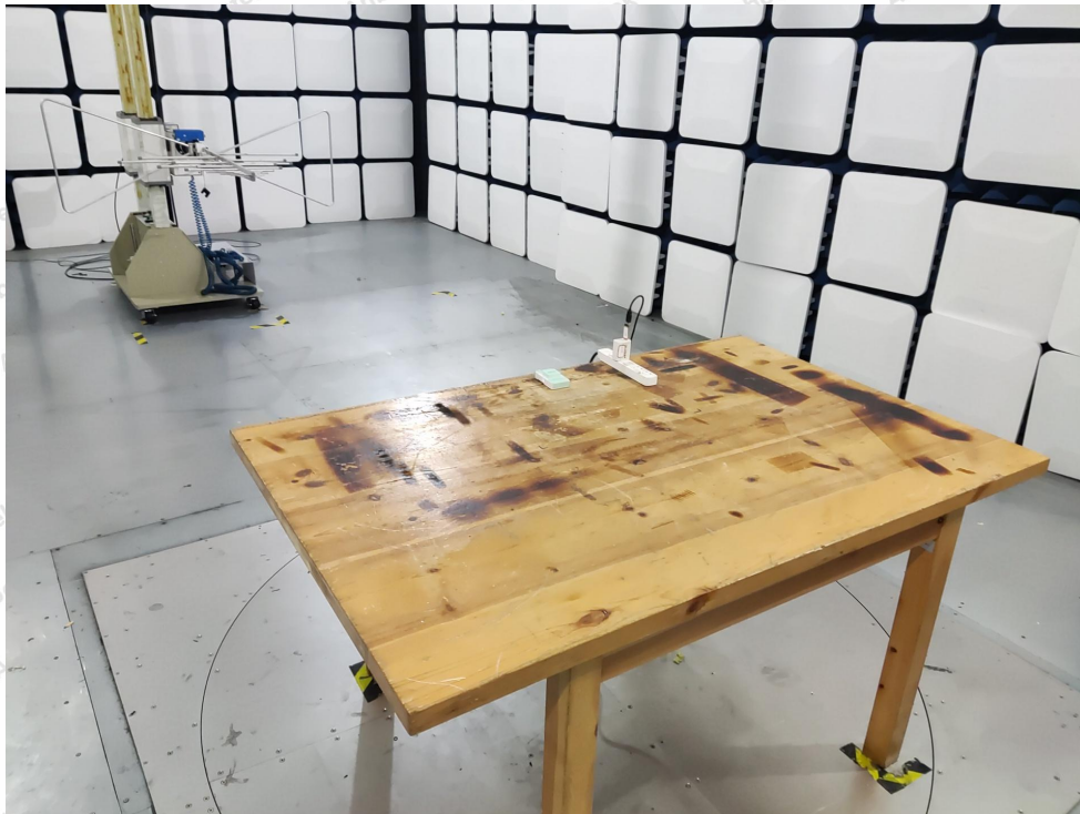
Photo of Radiation Emission Test
