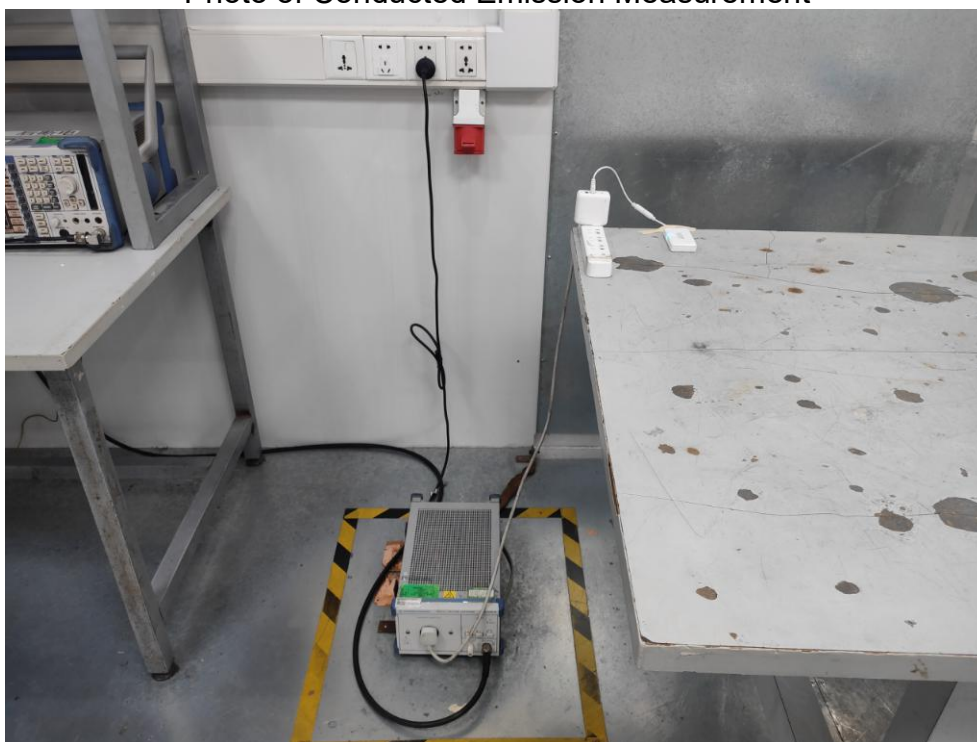
FCC ID: 2ARNO-VAP11AC Photo of Conducted Emission Measurement
