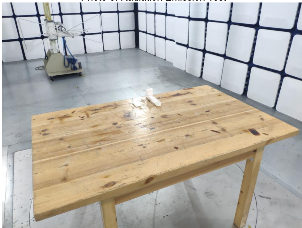
Photo of Radiation Emission Test
