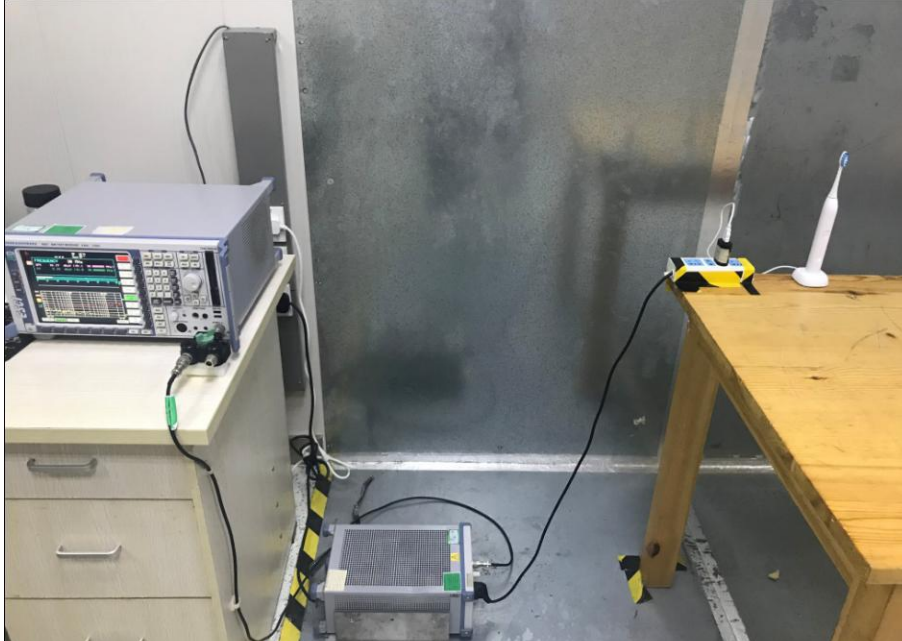
Radiated Spurious Emissions Test Frequency From 9kHz-30MHz
