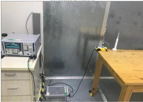
Radiated Spurious Emissions Test Frequency From 9kHz-30MHz
