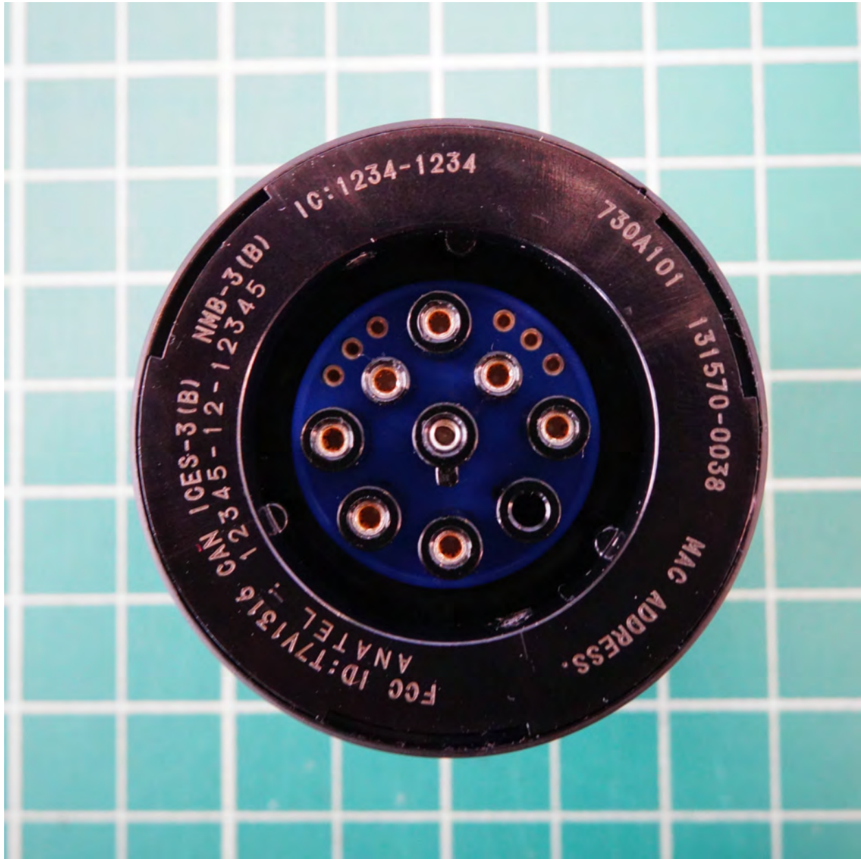
Picture 3 - Detailed view of FieldView Drive 2 enclosure bottom, including view of the J1939 connector and prototype markings. These markings do not reflect what will be used on the final product.
