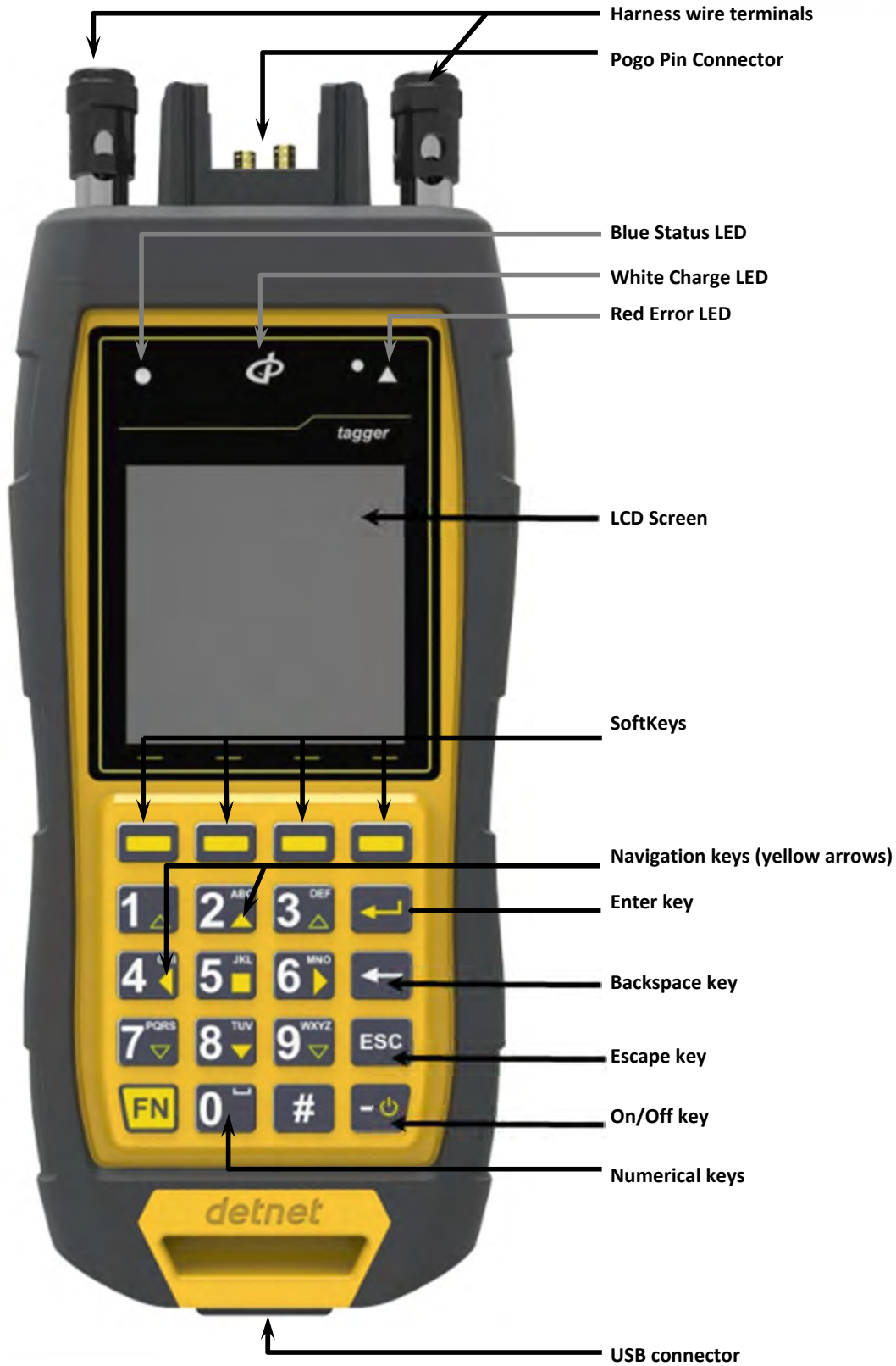
Figure 4: CE4 Tagger Component Identification
