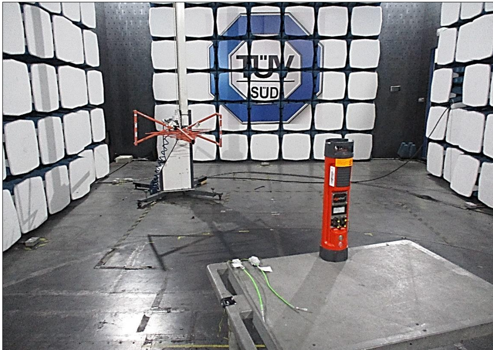
Figure 14 - Test Setup - 30 MHz to 1 GHz
