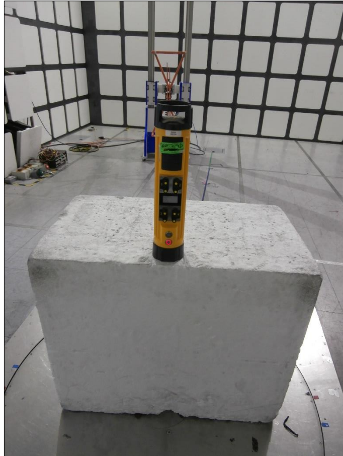
Figure 20 - Test Setup - 30 MHz to 1 GHz
