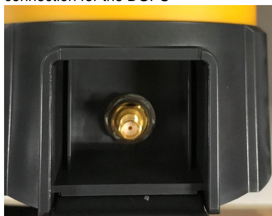
Photo 6: Base of unit showing antenna connection for the DGPS
