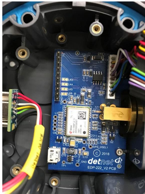
Photo 4: Close up view of DGPS PCB
