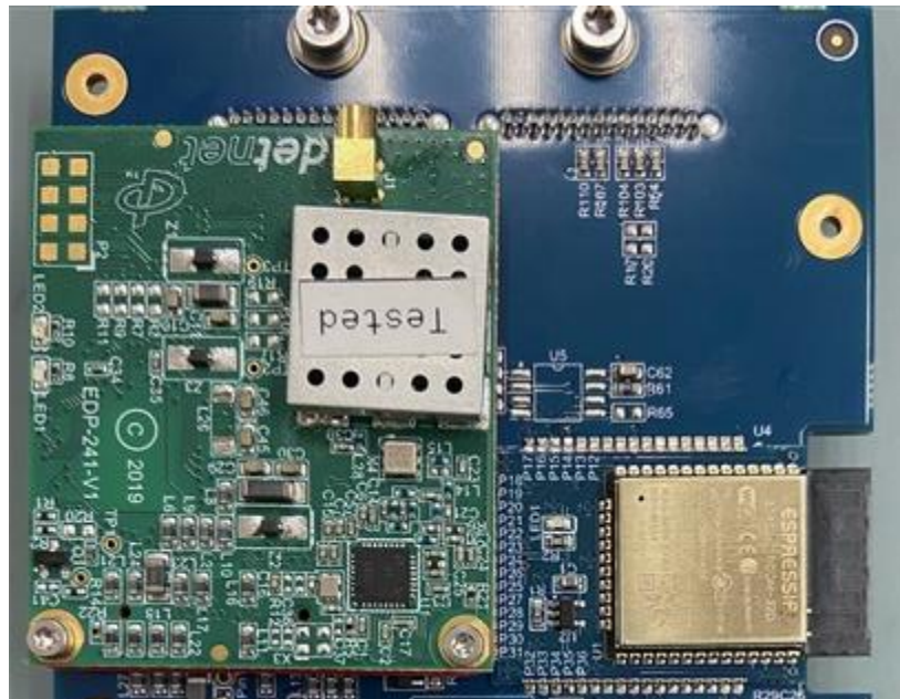
Photo 13: Close up of RF Module and WiFi Module
