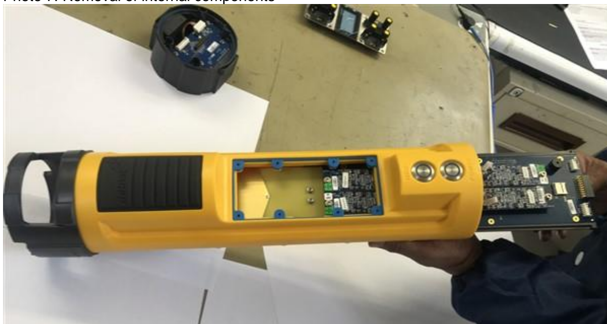
Photo 7: Removal of internal components
