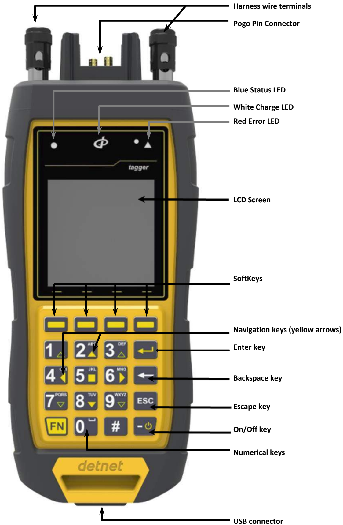
Figure 5: CE4 Tagger Component Identification
