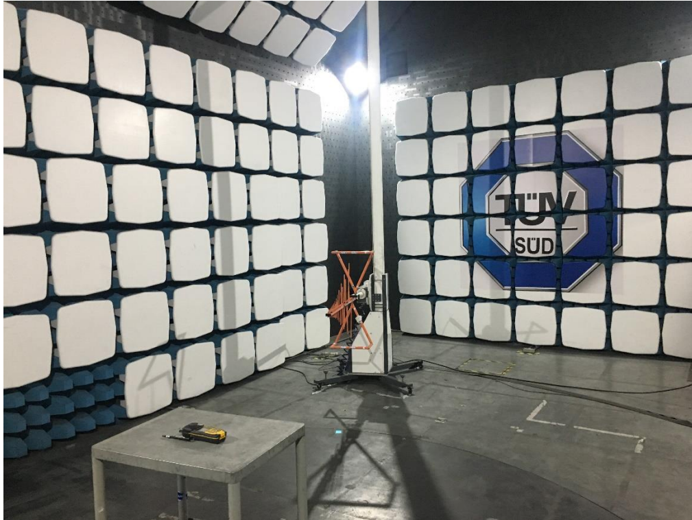
Figure 1 – Test Setup- 30 MHz to 1 GHz, X Orientation
