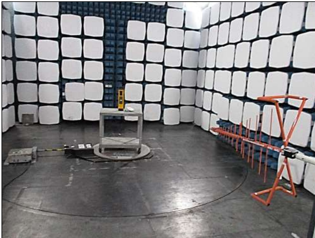
Figure 32 - Test Setup - 30 MHz to 1 GHz -Commander
