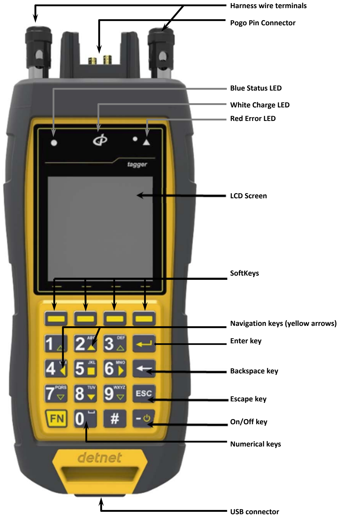
Figure 5: CE4 Tagger Component Identification
