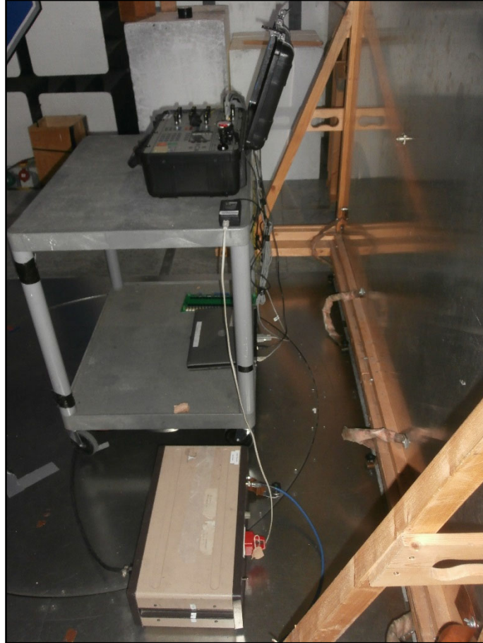
Figure 1 – Conducted Disturbance at Mains Terminals (FCC Part 15B, ICES-003 and RSS-GEN)
