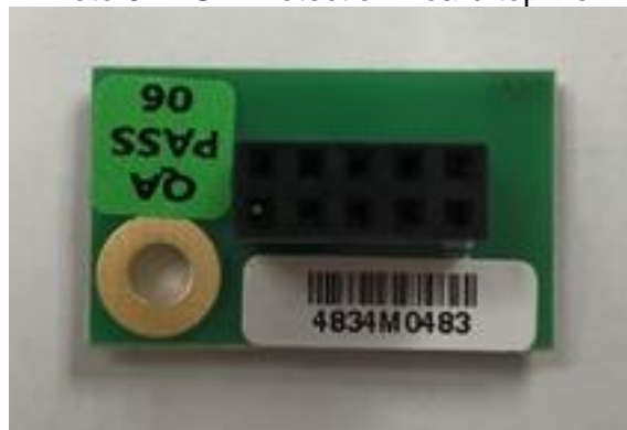
Photo 3: ESD Protection Board top view
