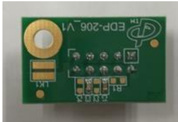
Photo 4: ESD Protection Board bottom view
