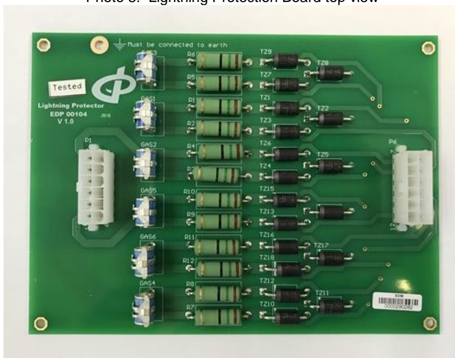
Photo 5: Lightning Protection Board top view
