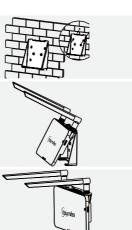
Fix DTU-Pro-S/DTU-Pro-S-C to the bracket's lower buckle gently until you hear a click. Please make sure that the antennas are vertical to the wall.
