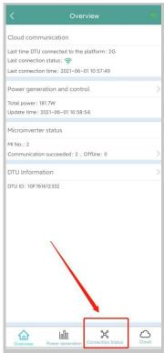
2. On this page, you can check the signal strength between the DTU and each microinverter. Tap the signal icon to enter the respective microinverter page (signal quality is constantly refreshing).
