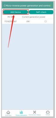
3. You can add microinverter via "Automatic Search" or typing in the microinverter ID or scanning the ID.
