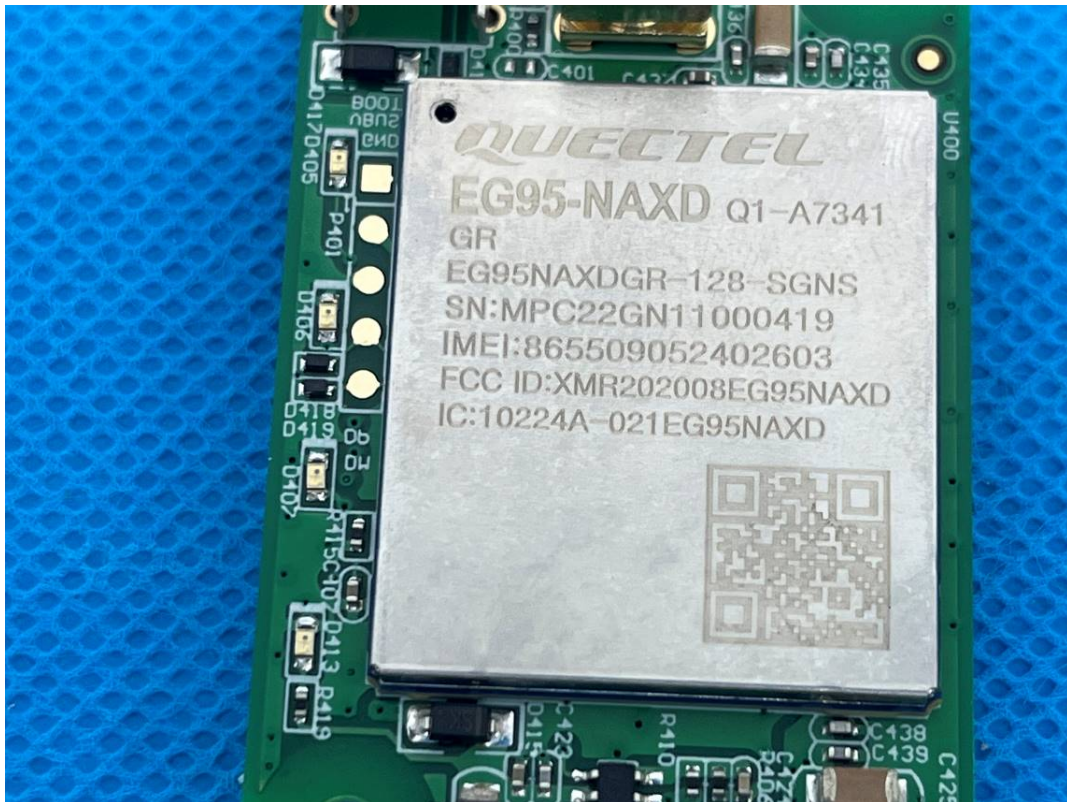
WWAN Module FCC ID: XMR202008EG95NAXD, IC: 10224A-021EG95NAXD
