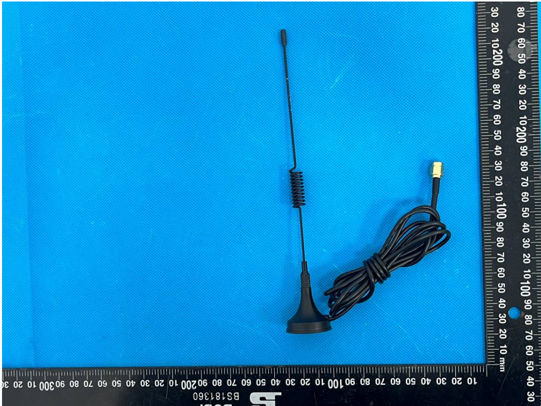
2.4G SRD Antenna(The 2.4G SRD has the same antenna as the WWAN)
