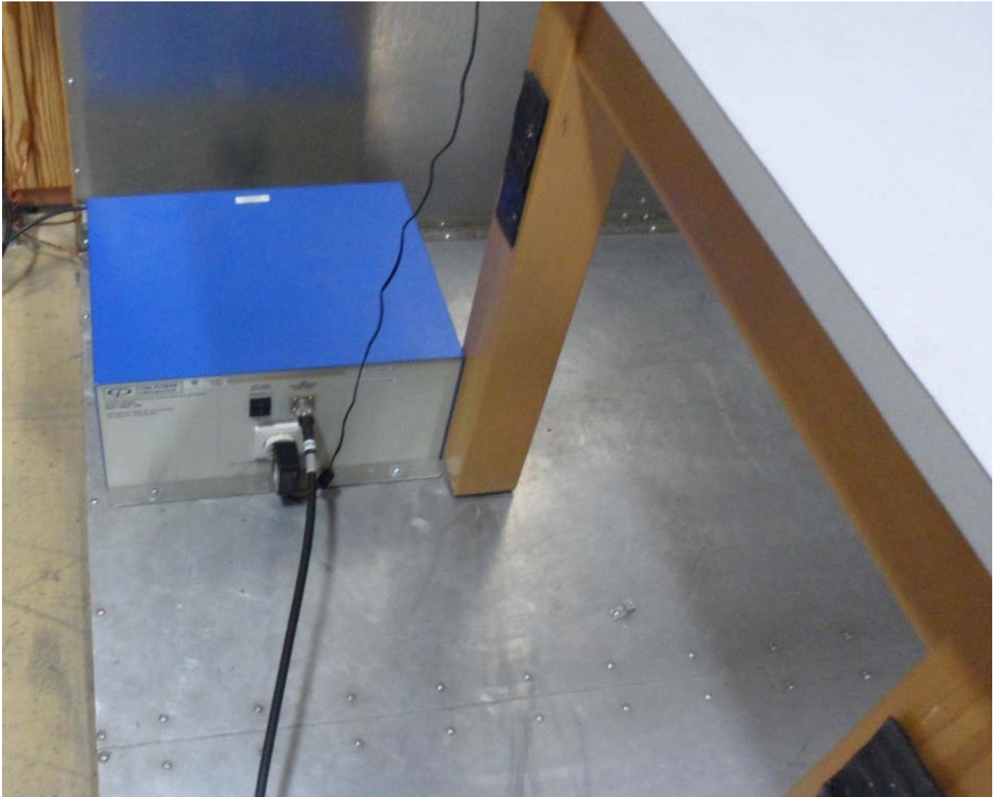
Figure E23.4 – Setup Photo – Power Line Conducted Measurements
