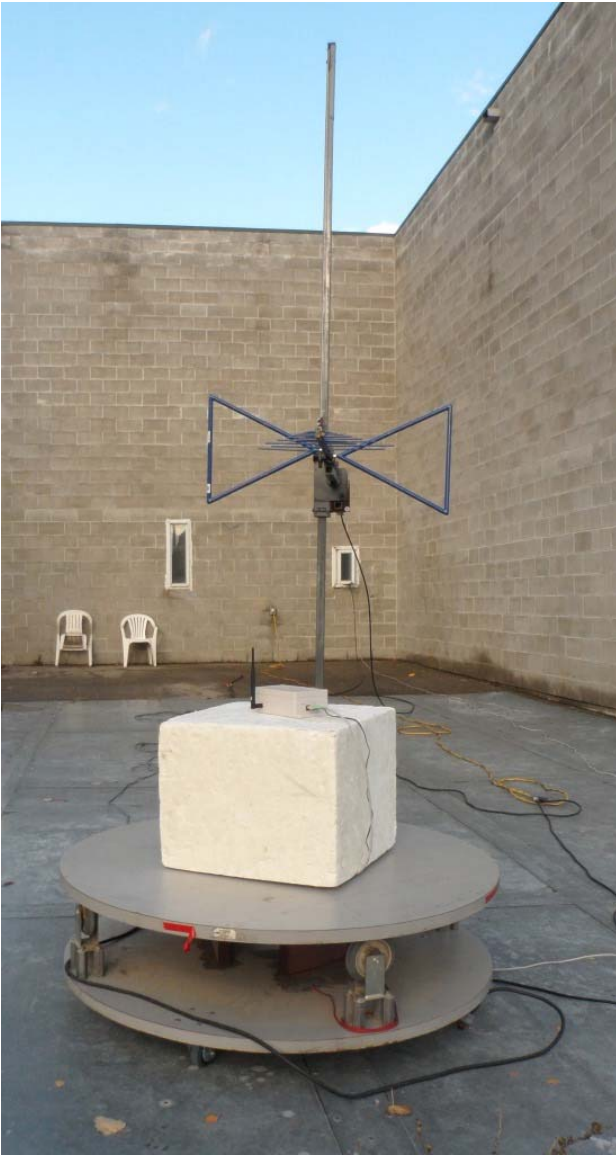
Figure E23.2 – Setup Photo – OATS Radiated Measurements 30MHz – 1000MHz Horizontal
