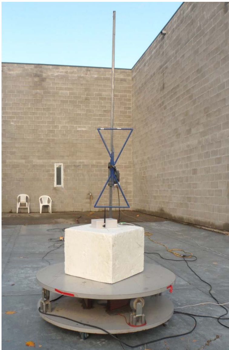
Figure E23.3 – Setup Photo – OATS Radiated Measurements 30MHz – 1000MHz Vertical
