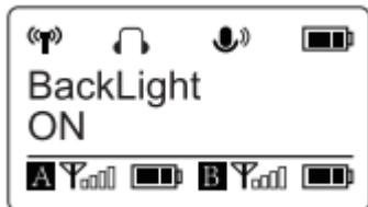
Set backlight: Set the background LED light to ON or Delay by 60, 30, or 10 seconds. Default setting is "Delay 30s."
