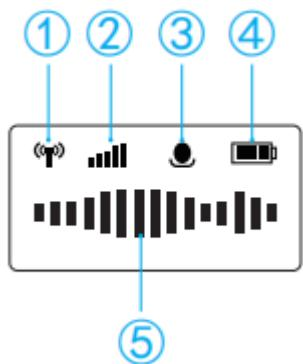
Home screen: If no operation is performed for 20 seconds on the other screens, the display will automatically return to the home screen.
