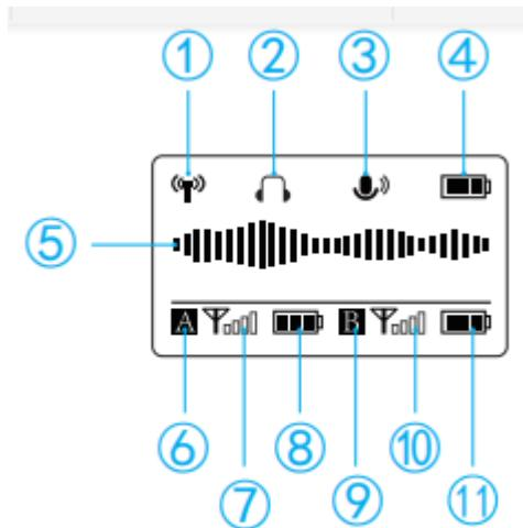
Home screen: If no operation is performed for 20 seconds on the other screens, the display will automatically return to the home screen.
