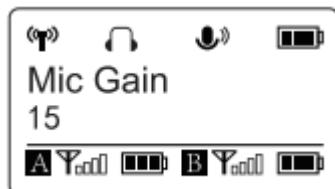
*MIC GAIN:* Adjust the external microphone's gain level (0-19). Default is "15"
