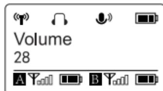
*Set output volume:* Set the volume of output audio within the range of 0 to 31. The setting is retained even after the power is turned off.
