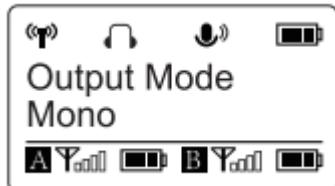
*Output mode:* The output mode can be set to mono or stereo. When the output mode is in mono, the audio from the left and right channel will be mixed. When in stereo, receiver A's and receiver B's audio output will be separated to the left and right of the stereo output.
