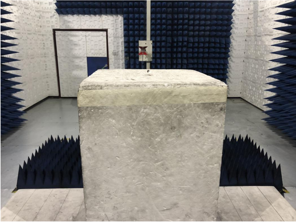
RADIATED EMISSION TEST SETUP ABOVE 1GHZ
