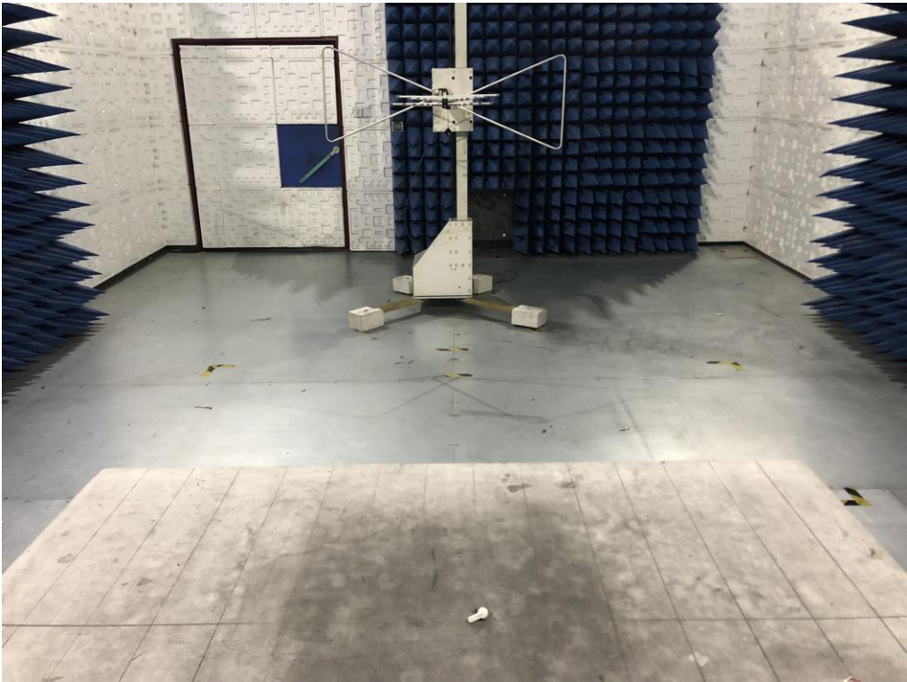
RADIATED EMISSION TEST SETUP ABOVE 1GHZ
