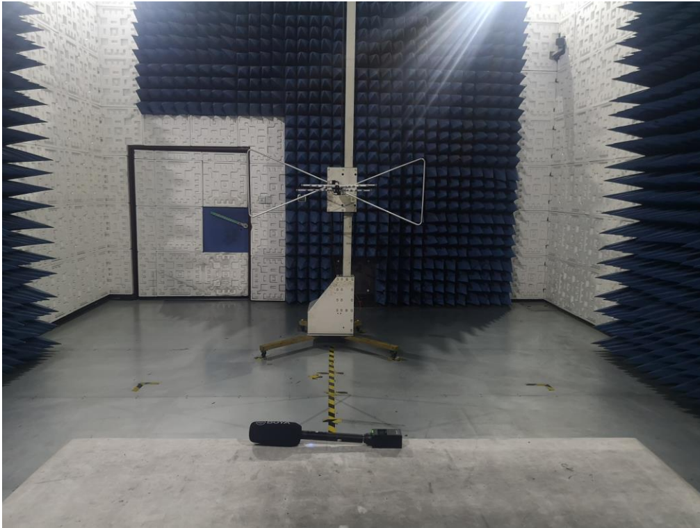
RADIATED EMISSION TEST SETUP ABOVE 1GHZ
