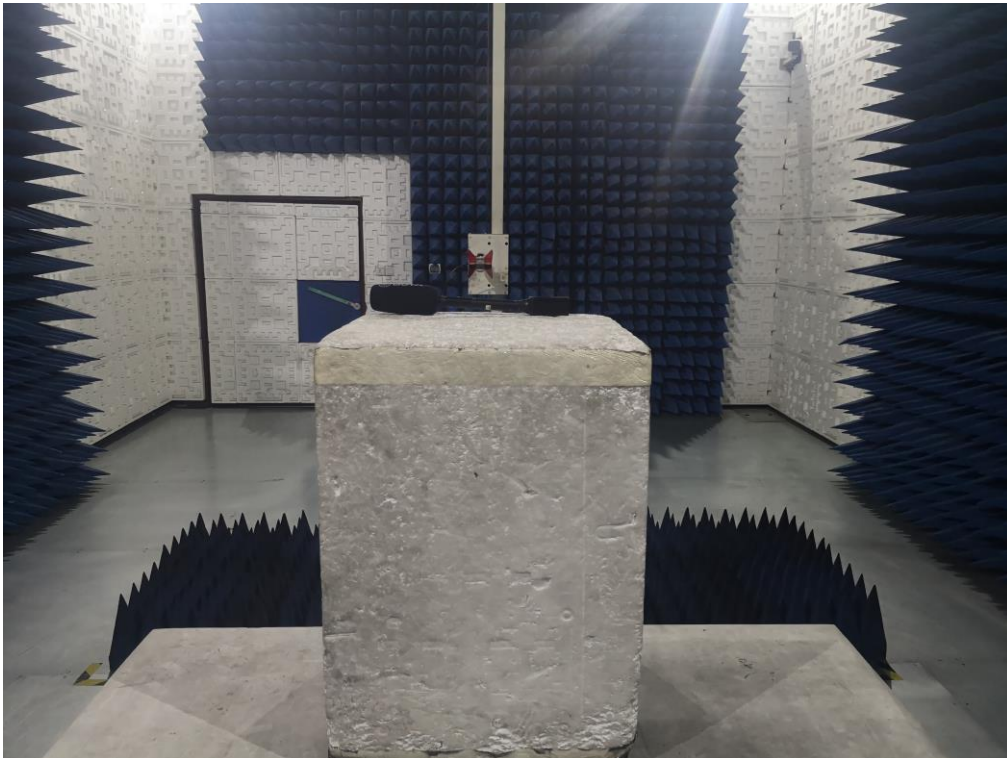
RADIATED EMISSION TEST SETUP ABOVE 1GHZ
