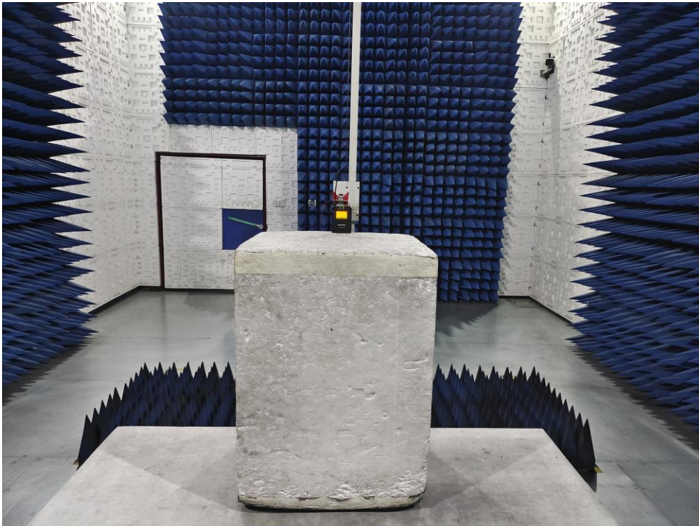
RADIATED EMISSION TEST SETUP ABOVE 1GHZ
