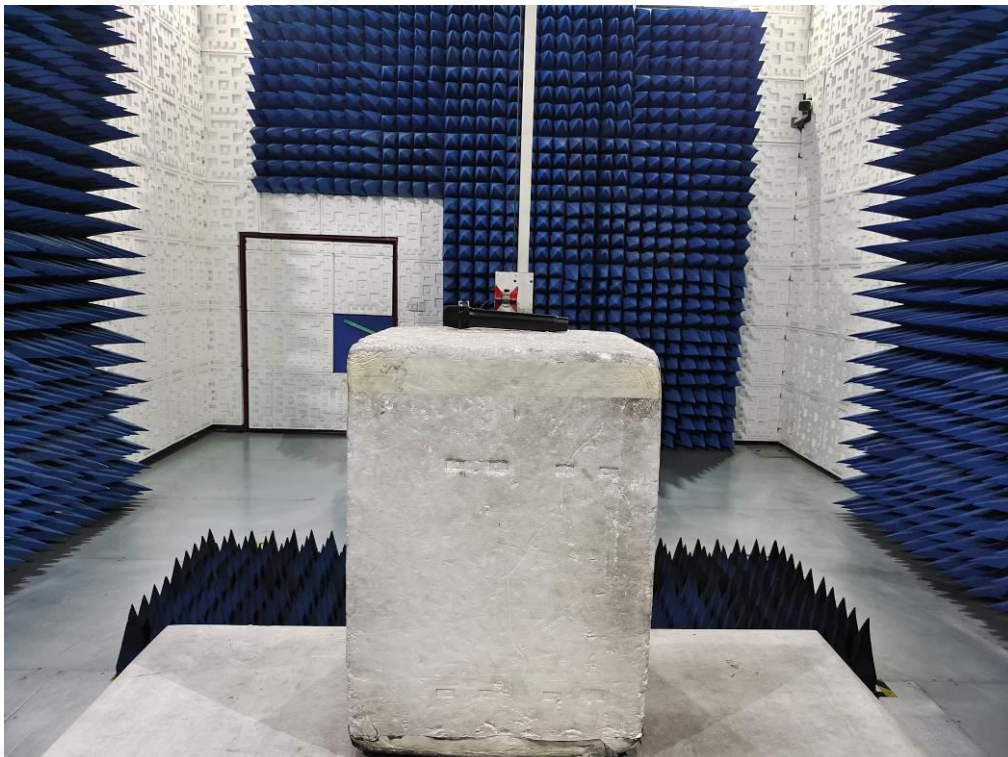
RADIATED EMISSION TEST SETUP ABOVE 1GHZ
