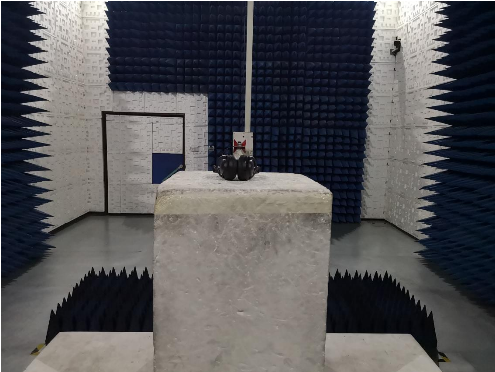
RADIATED EMISSION TEST SETUP ABOVE 1GHz
