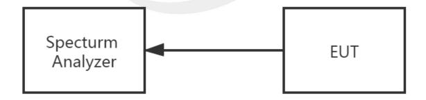
The EUT which is powered by the DC Power, is connected to the Spectrum Analyzer; the RF load attached to the EUT antenna terminal is 50 Ohm; the path loss as the factor is calibrated to correct the reading. Make the measurement with the spectrum analyzer's resolution bandwidth(RBW) = 100 kHz. In order to make an accurate measurement, set the span greater than RBW.
