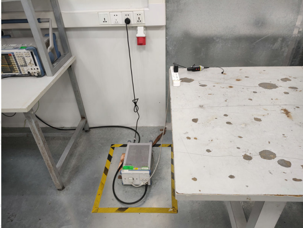
Photo of Conducted Emission Measurement
