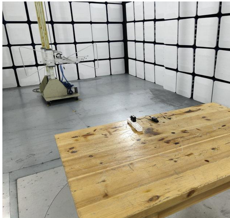
Photo of Radiation Emission Test
