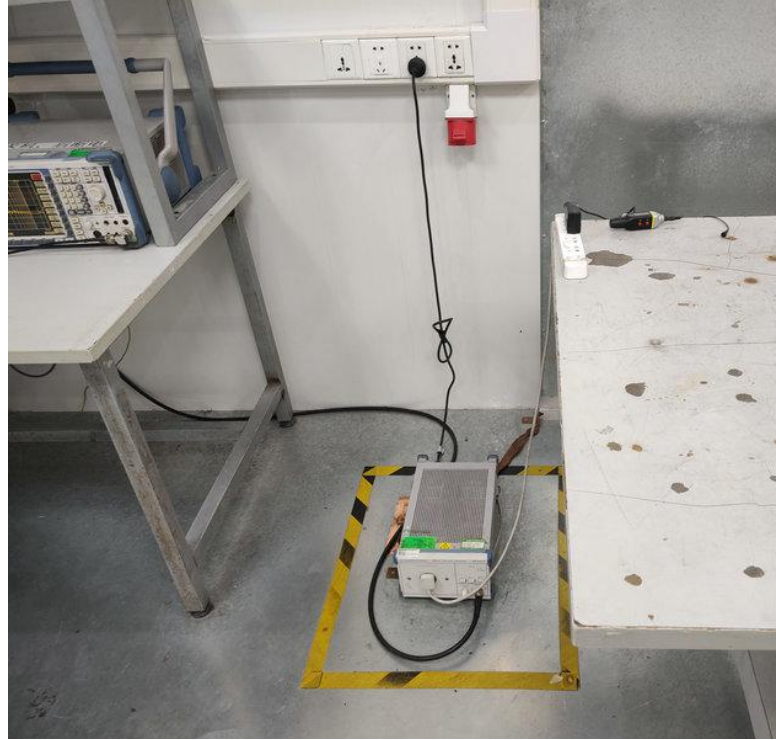
Photo of Conducted Emission Measurement
