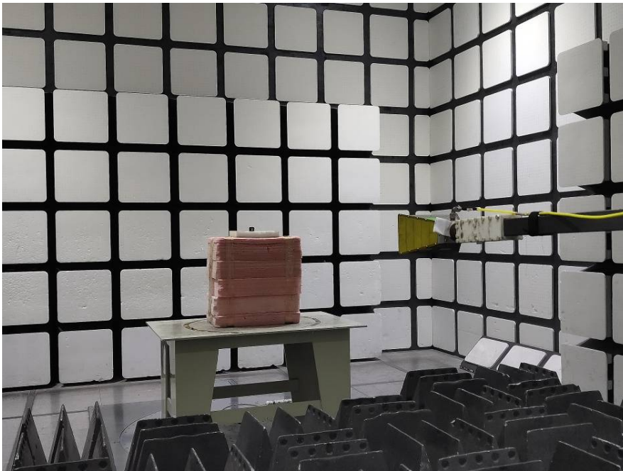
Radiated Emissions View (Above 1 GHz)
