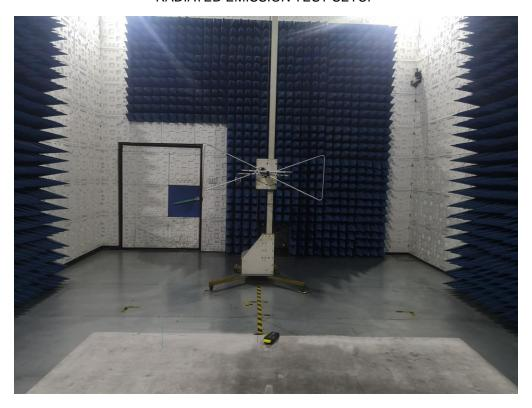
RADIATED EMISSION ABOVE 1G TEST SETUP
