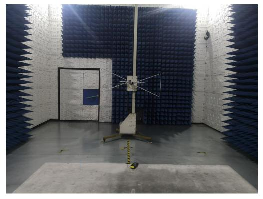
RADIATED EMISSION ABOVE 1G TEST SETUP
