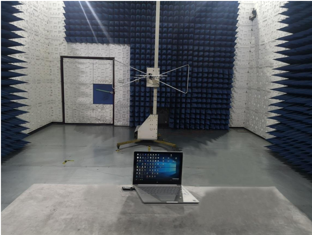
RADIATED EMISSION TEST SETUP BELOW 1GHZ
