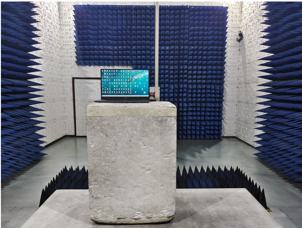
RADIATED EMISSION TEST SETUP ABOVE 1GHZ
