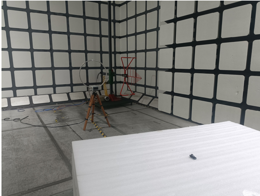
Radiated Emissions View (9 kHz- 30 MHz)
