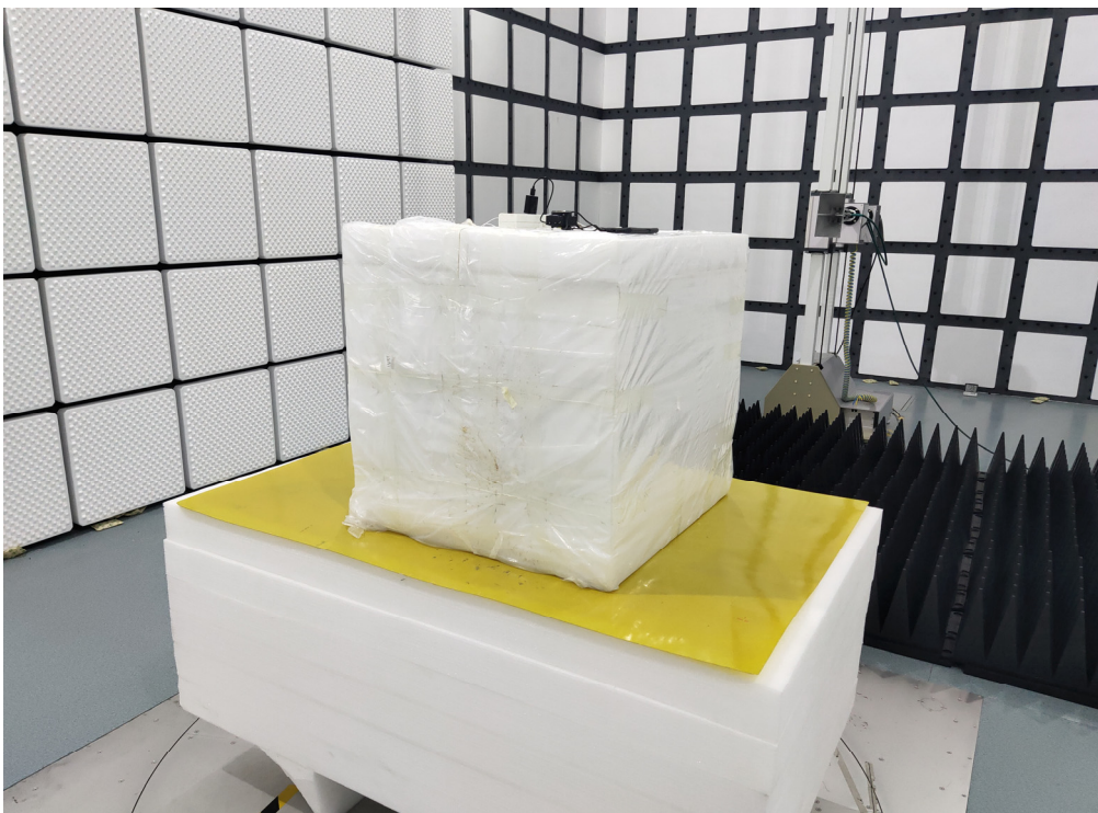
Photo of Radiated Emission Measurement (Above 1G)
