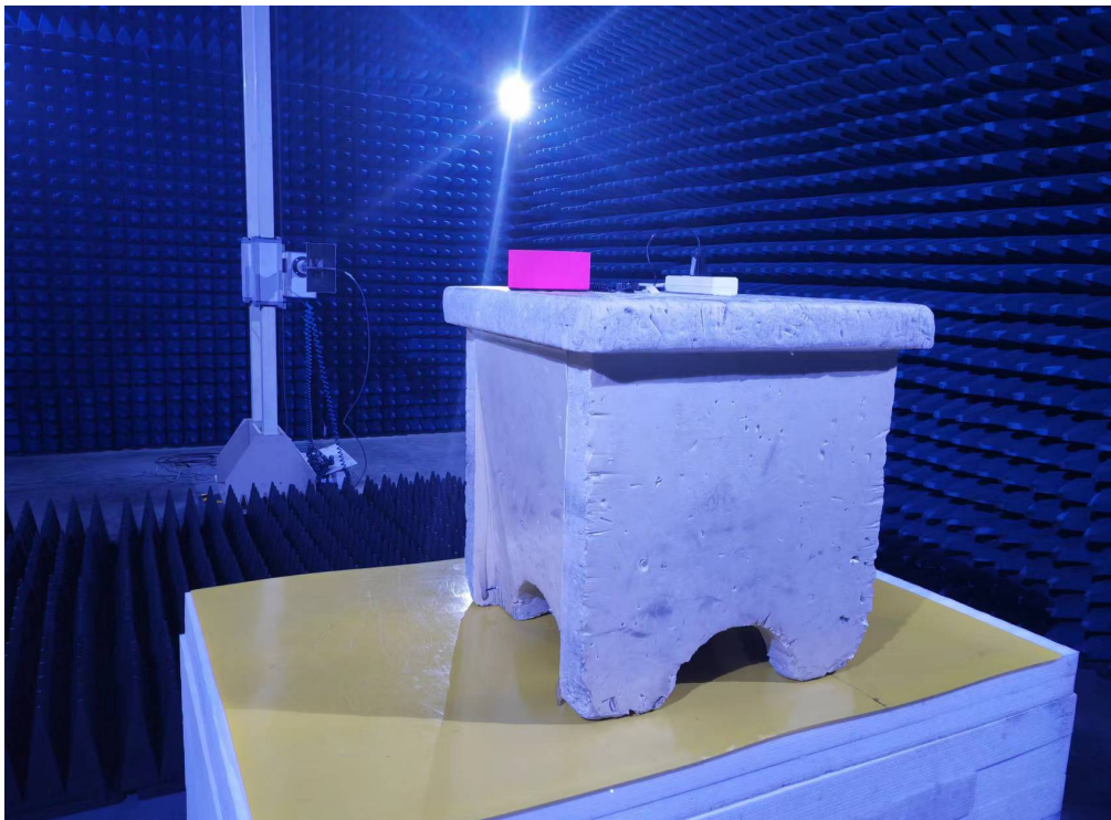
Photo of Radiated Emission Measurement (Above 1G)
