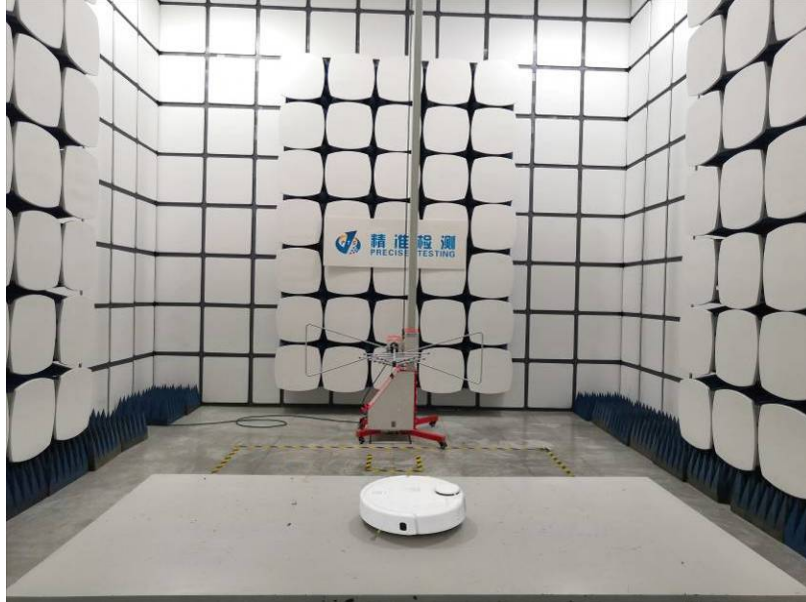
Radiated Spurious Emissions Test Frequency From 30MHz-1000MHz
