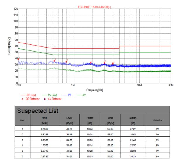
Remark: Transd = Cable lose + Antenna factor - Pre-amplifier; Margin = Limit – Level
