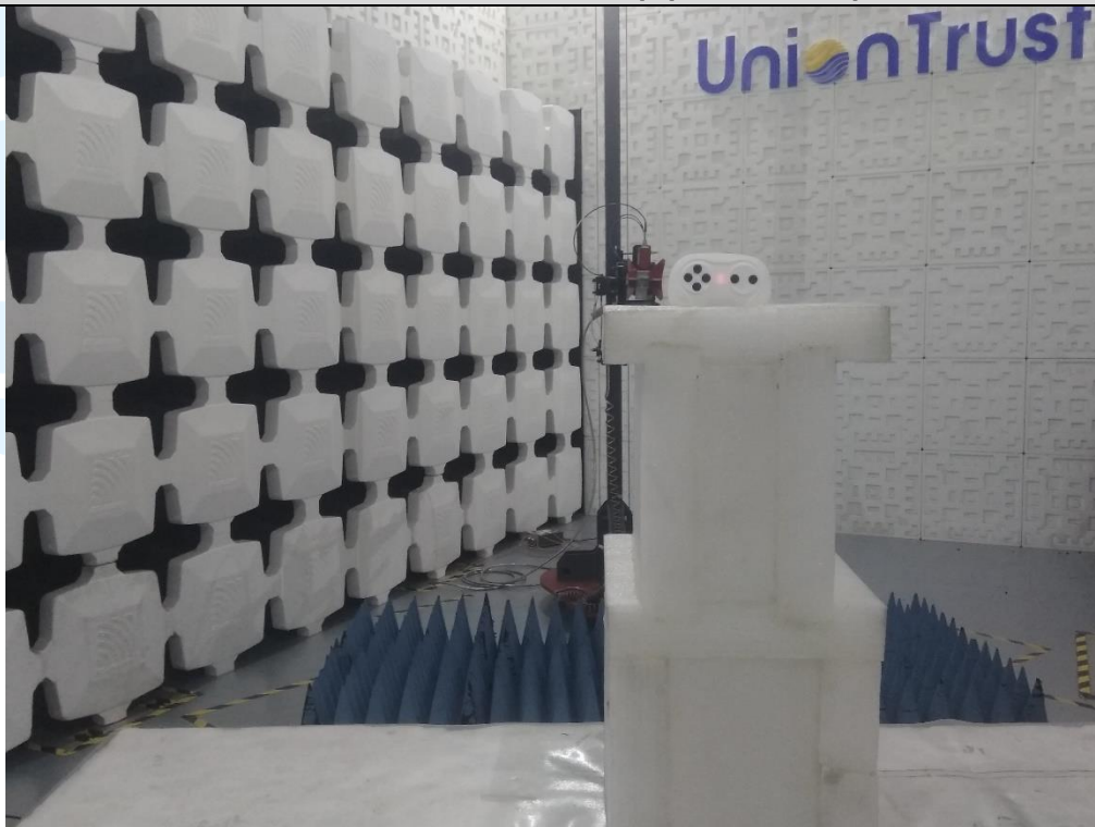
Radiated emission Test Setup (Above 1 GHz)
