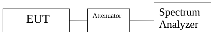
Figure 3. Block Diagram, Maximum Conducted Output Power Test Setup
