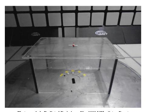
Photograph 4. Radiated Emissions, 30 – 1000 MHz, Setup Front
