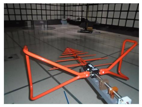
Photograph 5. Radiated Emissions, 30 – 1000 MHz, Setup Antenna
