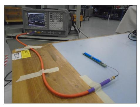
Photograph 1. Occupied Bandwidth Setup
