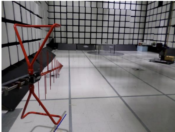
Figure 2: Radiated Emissions - 30MHz-1000MHz - Setup Antenna View
