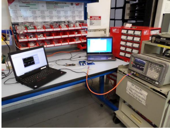
Figure 1: Conducted Spurious Emissions Setup Photo
