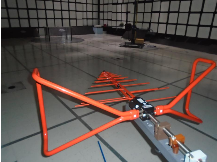
Photograph 7. Radiated Emissions Setup, 30 – 1000 MHz, Antenna
