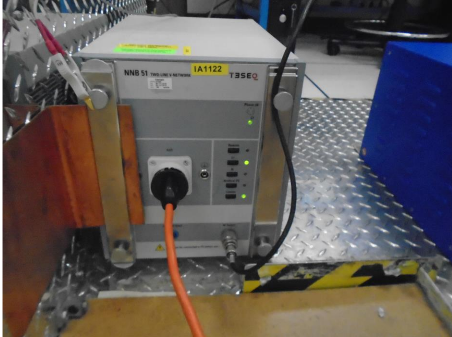
Photograph 3. Conducted Emissions, LISN Connection
