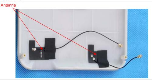
The antenna is IPEX antenna. The best case gain of the ant1 and ant2 is 2dBi,MIMO is 5.01dBi.
