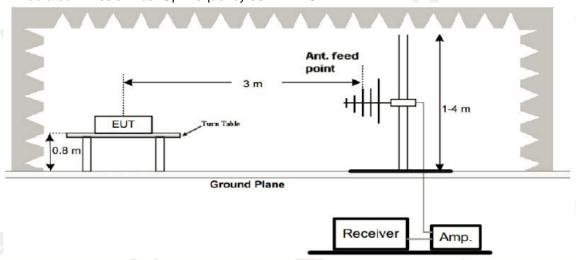
3. Radiated Emission Test-Up Frequency Above 1GHz
