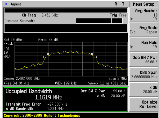
20dB Bandwidth plot on channel 39 (2Mbps)
