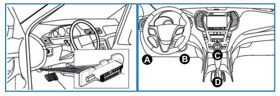
For the in-car installation, connect MocBox to the OBD port of the vehicle and hide and fix the MocBox behind the plastic panels of the dashboard as shown in the picture. As for the detailed installation process or installation in other kinds of vehicle, please contact MoC Team for further documentation.
