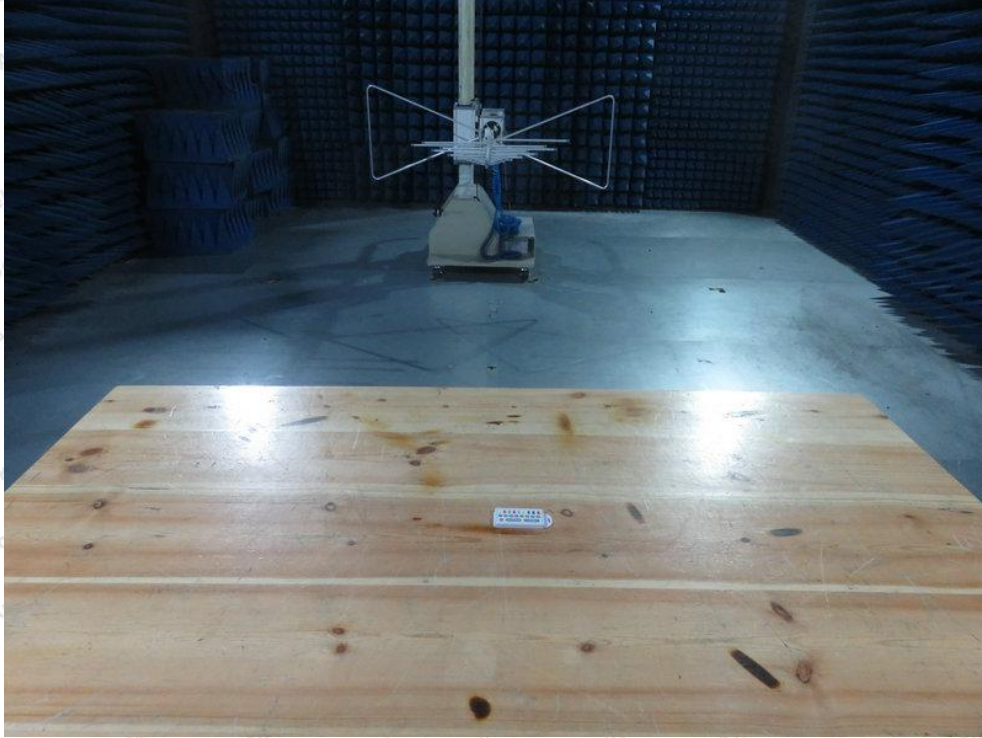
Photo of Radiation Emission Test
