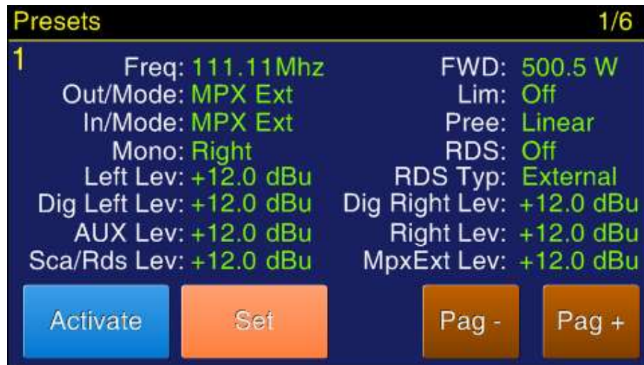
Fig. 31: Presets panel of an inactive memory
