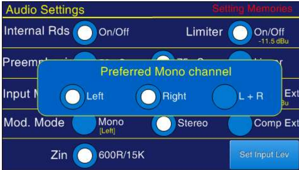
Fig. 12: Modulation mode settings
