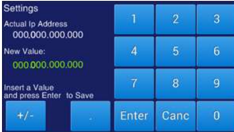
Fig. 15: Setting LAN Ip Address
