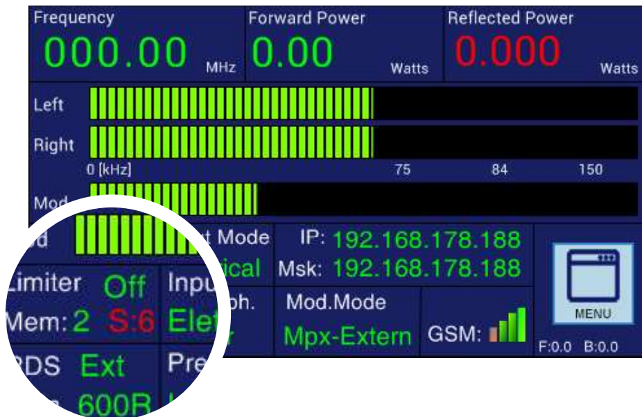
Fig. 29: Zoom of the active memory indication in the main screen
